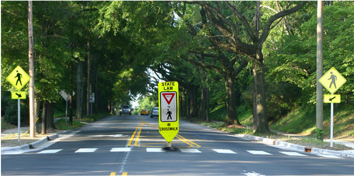
Figure 23. Example of Pedestrian Warning Signs
